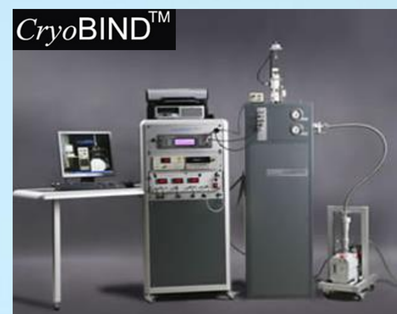
The commercial CryoBIND high-sensitivity magnetic ac susceptibility measuring device is fully developed at the Institute of Physics. http://www.cryobind.com
