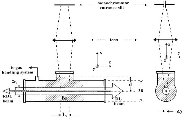
**Fig. 1.** Experimental arrangement; DL: diode laser, RDL: ring dye laser,  $d$ : length of the optical path through the layer of non-excited barium vapour,  $L_z$ : length of the observed fluorescence slab defined by the height of the monochromator entrance slit and imaging ratio (1:2),  $\Delta y$ : width of the observed fluorescence slab defined by the monochromator entrance slit width,  $2r_0$ : diameter of the pump laser beam,  $2R$ : heat-pipe diameter.
