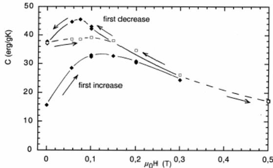
**Figure 3.** Magnetic field dependence of  $c_p$  of o-TaS<sub>3</sub> at 100 mK.
