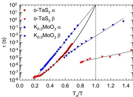
**Figure 4.** Temperature dependence of the relaxation times of two processes observed in K<sub>0.3</sub>MoO<sub>3</sub> and o-TaS<sub>3</sub>. The temperature scale is renormalized to  $T_g$  equal 23 K and 50 K respectively.
