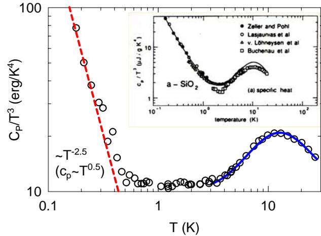
**Figure 1.** Heat capacity  $c_p$  of  $K_{0.3}MoO_3$  presented as  $c_p/T^3$ . Solid line is the fit to the gapped phason model and the dashed line is the low temperature power-law contribution. Inset is corresponding plot for  $SiO_2$  glass.
