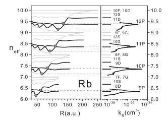
FIG. 3. Calculated  $^{3}\Sigma$  Rb\* – Rb Born-Oppenheimer excited state potential curves (left) and the relevant experimental line shapes (right) of the Rb 5S - nP (n = 9, 10, 11, 12) transitions. In contrast to Fig. 2, the energies are represented in terms of the effective principal quantum numbers  $n_{\rm eff}$ . The positions of the potential curves minima which produce the line satellites are labeled by gray circles.
