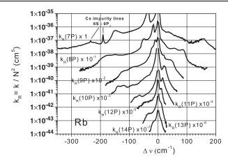
FIG. 1. The reduced absorption coefficients  $k_R(nP) = k(nP)/N_{\rm Rb}^2$  of the quasistatic wings of some Rb 5S-nP lines are plotted versus the wave number difference from the respective line centers. For better representation, the individual spectra have been multiplied by different factors of 10 as indicated.
