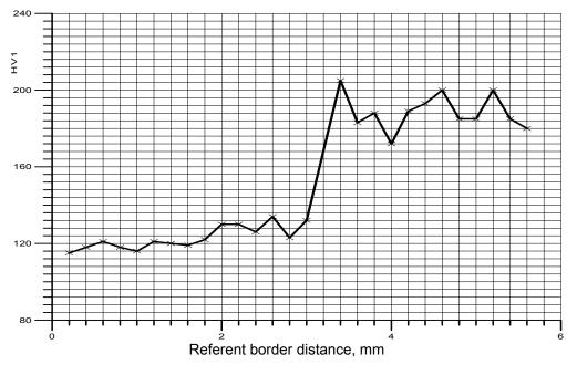
Figure 6. HV1 hardness on the 5 mm distance from the weld pass start (line D)
