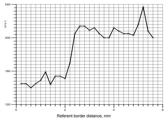
Figure 10. HV1 hardness on the 79 mm distance from the weld pass start (line C)
