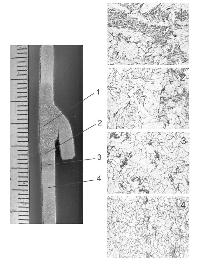
Figure 12. Macro and micro analysis of the welded joint on the weld start
