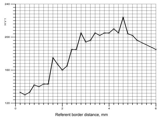
Figure 9. HV1 hardness on the 40 mm distance from the weld pass start (line E)
