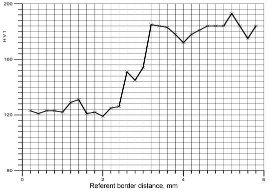
Figure 8. HV1 hardness on the 15 mm distance from the weld pass start (line B)
