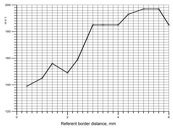
Figure 11. HV1 hardness on the 115 mm distance from the weld pass start (line F)
