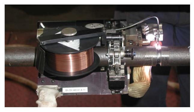
Figure 11. Detail of butt automatic orbital TIG welding pipes for steam boiler plants
