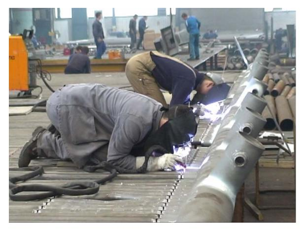
*Figure 3. Manual TIG butt welding of pipes on boiler chamber*
