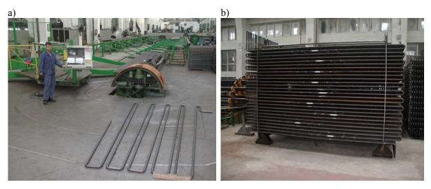
Figure 1. CNC-cold pipe bending machine (a) and prepared deformed pipes set (b).
