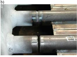
*Figure 2. Butt MMA pipe welding of membrane pipe panel–chamber with pipe connectors (nozzles) (a) and detail of joining location (b)*
