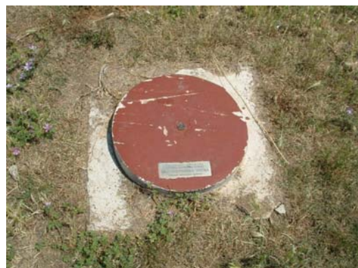
Figure 4: New gravity station monumentation
