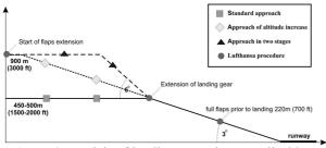
Figure 2. Models of landing procedures applicable at Zagreb Airport
