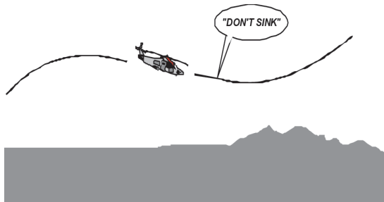
Fig. 4. Alert is triggered by the combination of Altitude (Pressure Alt) Loss Vs Clearance (Radio Alt)
