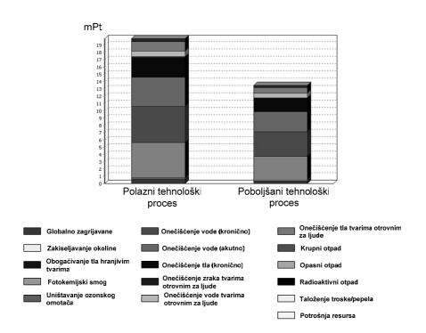
Figure 5 Comparison of the initial and improved technological processes [8]
