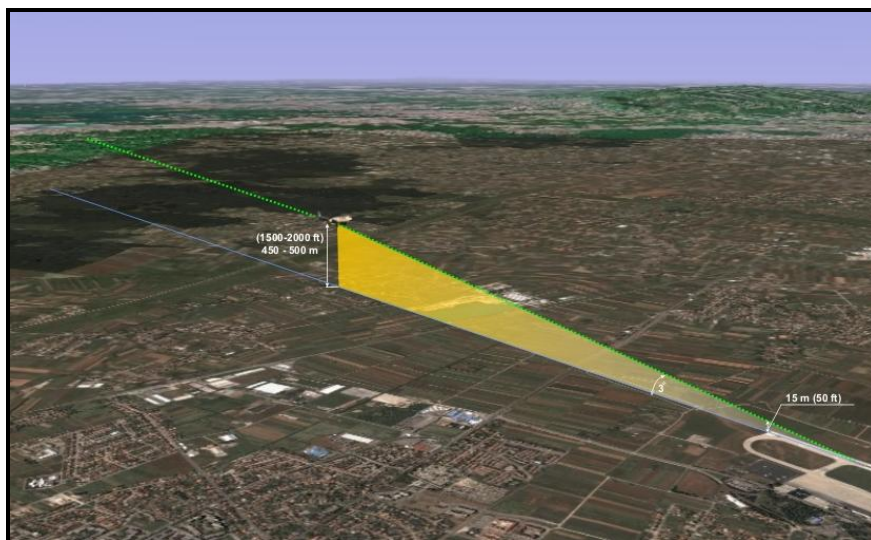
Figure 3: Standard landing procedure
