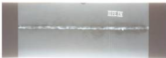
Figure 2. Radiographic film of welded joint with porosity (recorded by digital camera)
