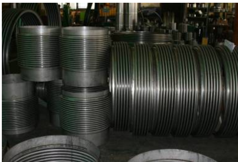
Figure 1. Bellow production in ĐĐ Kompenzatori d.o.o. factory
