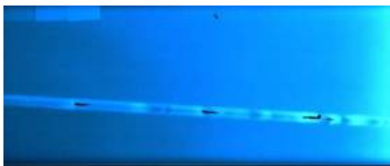
Figure 6. Example of scanned radiographic film with weld porosity (HP SCANJET 5500c)
