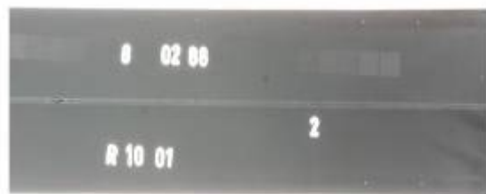
Figure 3. Radiographic film of welded joint with incomplete penetration (recorded by digital camera)
