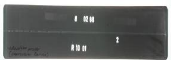
Figure 5. Example of scanned radiographic film with incomplete penetration of weld joint (MICROTEC SCANMAKER 9600 XL)
