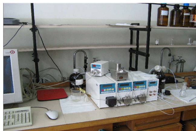
Fig. 1. Knauer K-501 pumps and Wellchrom DAD K-2700 detector at 215 nm.
