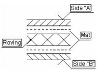
Figure 1. Schematic layout of reinforcement in the matrix of plates
