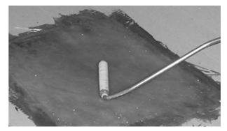
Figure 2. Production procedure by soaking and by pressing the air out (by hand roller)
