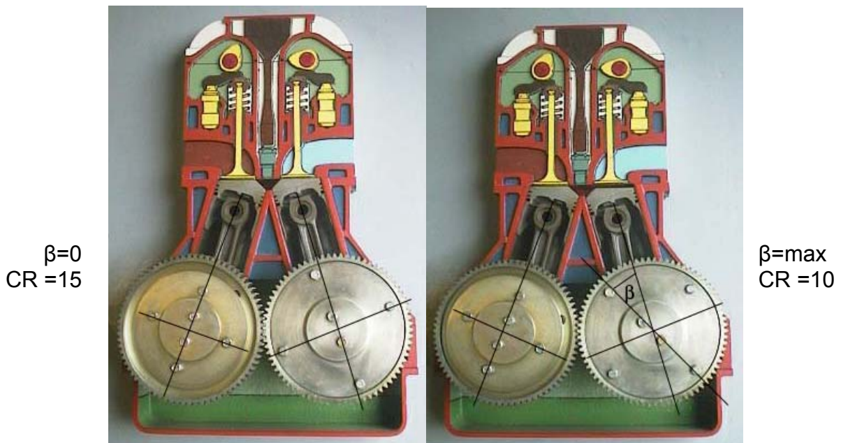
Figure 14 The “CVCR” engine with self - adjusting compression ratio
