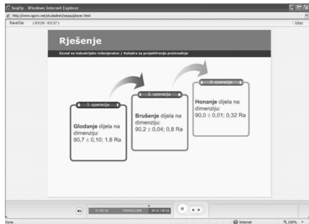
Figure 12 : Final solution of sequencing operations
