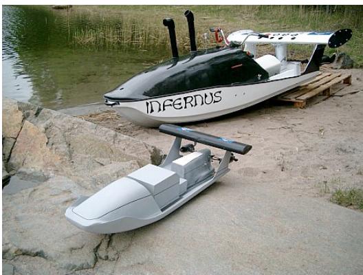
Fig. 3 Infernus, the high-speed craft with underwater capabilities (2004)
