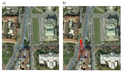
**Figure 2. Recorded GPS track (a) and actual PT vehicle position (b)** Source of orthophoto: Croatian State Geodetic Administration
