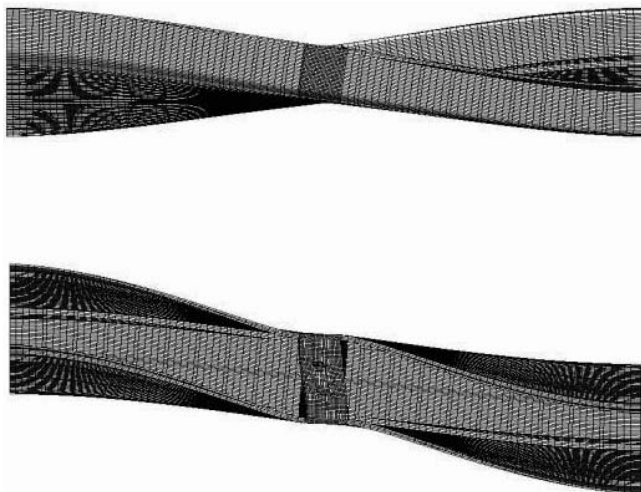
Figure 20 Deformation of segmented pontoon, lateral and bird's-eye view Slika 20 Deformacije segmentnog pontona, bočni i ptičji pogled
