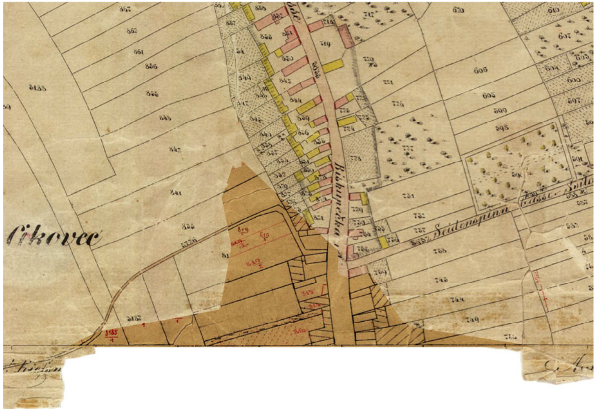
Figure 10: Visible discrepancies between the map A and moved and rotated the triangular part of the map B.
