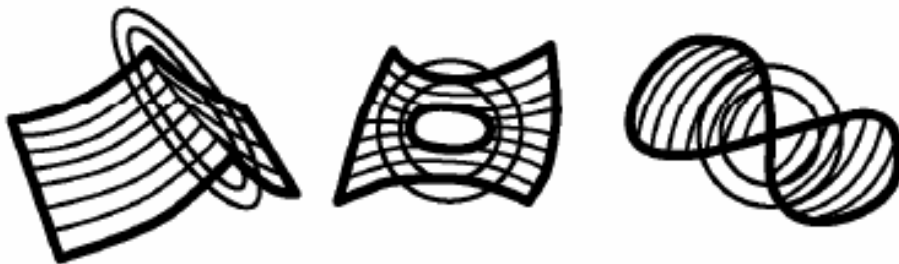
Figure 14 - Examples of point sets in space, which are not surface elements (here a double circle means "not smooth") (INTERLIS Version 2 - Reference Manual, 2006.)
