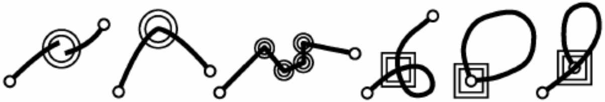
Figure 8 – Examples of planar sets not being curve segments (a double circle indicates „not smooth“ and a double square „not injective“) (INTERLIS Version 2 - Reference Manual, 2006.)
