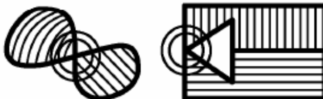
Figure 16 - Examples of planar point sets that are not surfaces (a double circle marks a "singular point") (INTERLIS Version 2 - Reference Manual, 2006.)
