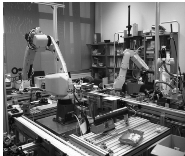
Fig. 2 The environment used for model developing and testing. It contains six axes robots, assembly line with stopping places, vision systems, optical, laser and capacitive sensors, parts to be assembled along with pallets and product carriers.
