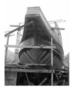
Figure 2. Building site and wooden structure of galleon 'Tirena'
