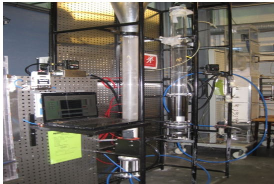
Figure 1: Experimental set-up: fluidized bed with pressure reduction valve, digital flow controller, pressure sensors.
