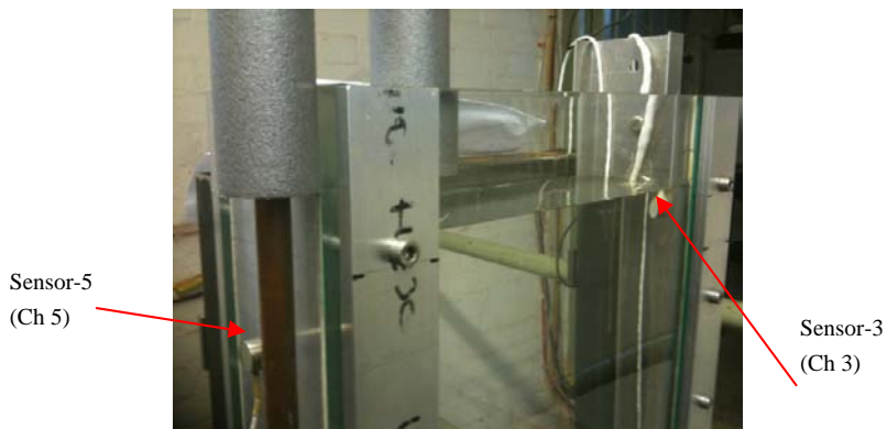
Figure 3: AE sensors mounted at the top (free surface) of bubble rig to detect the emission of bubble burst.
