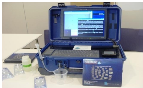
Fig. 3. Flow Cytometer exhibit by Fluid Imaging Co. on GloBallast R&D Forum in Istanbul, Oct., 2011. [7]
