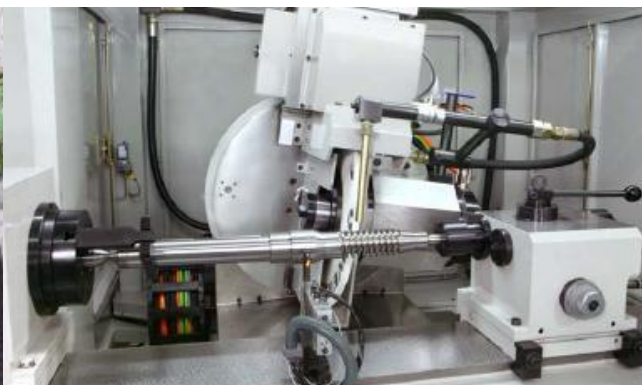
Figure 1b. Work zone of a grinding machine for machining of short threaded profiles
