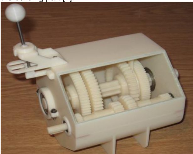
Figure 6. Assembled prototype of FDM gearbox
