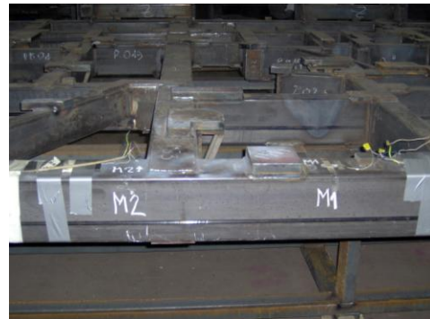
Figure 6. Strain gauges at the construction 1
