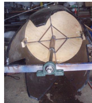
Figure 3. Installation of reinforcement and centring the front part
