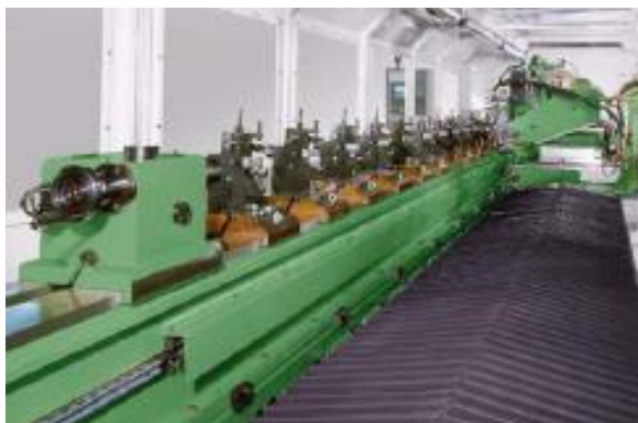
Figure 1a. Grinding of long lead screws with steady rests
