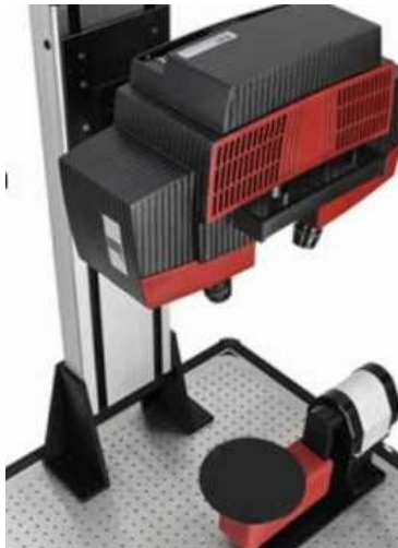
Figure 1. Atos III Triple Scan from GOM
