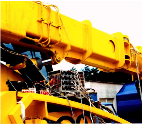
Figure 3. Data Logging and Processing Equipment
