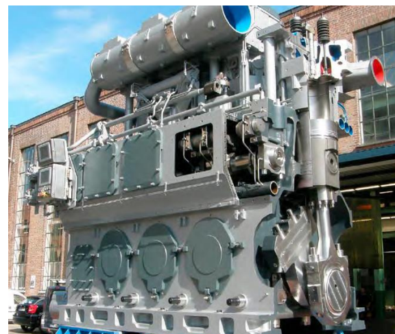
Figure 2. Large medium speed IC engine MAN Diesel 48/60CR [4]
