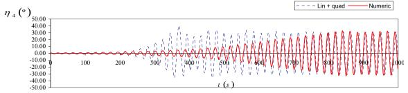
Figure 8-4. Time traces comparison of roll responses between equivalent linear damping by direct calculations and linear + quadratic model for test No. 304.
