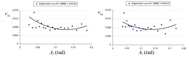
Figure 7-13. Linear + quadratic + cubic model for decay test "DECAY\_TEST\_GM1\_ U=0 knots" for both runs (Test 1 and Test2)
