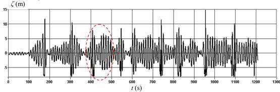
Figure 8-29. Wave elevation segment that enable parametric rolling.
