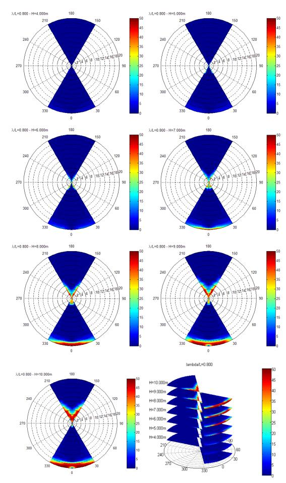
Figure 5-20. Numerical evidence with 2D and 3D polar plots (GM1) of parametric rolling with  $T_W = 11.59 \text{ s.}$
