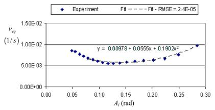
Figure 7-3. Linear + quadratic + cubic model for decay test 302
