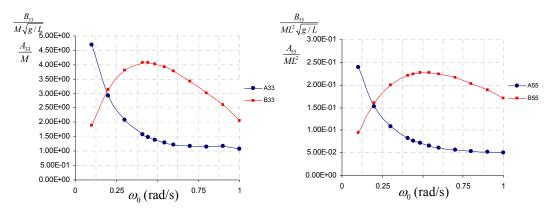
Figure 3-11. Variations of the hydrodynamic added mass and damping coefficients in heave and pitch depending on the various encounter frequencies
