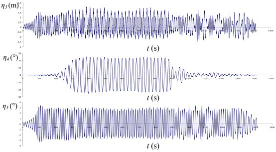
Figure 6-17. Development of parametric rolling in experiments with regular waves ( $H_W = 8 \text{ m}$ ,  $T_W = 12.95 \text{ s}$ , speed 8 knots)
