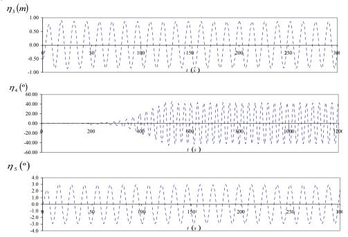
Figure 5-2. Development of parametric rolling in regular waves ( $H_W = 6 \text{ m}$ ,  $T_W = 12.95 \text{ s}$ , speed 7 knots)
