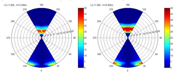
Figure 5-16. Numerical evidence with polar plots (GM1) of parametric rolling for ( $H_W = 5 / 6$  m,  $T_W = 12.95$  s).
