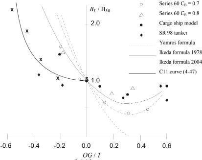
$\left(\frac{OG}{T}\right)$  given for calculating the lift damping coefficient Figure 4-10. Curve of the new function f
