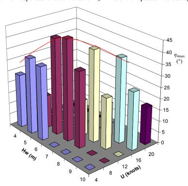
Figure 5-10. Quantitative validation of regression fit for the occurrence regions of parametric rolling
