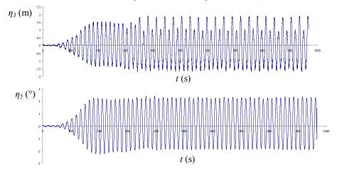
Figure 8-9. Heave and pitch motions in experiment (test No. 312)
