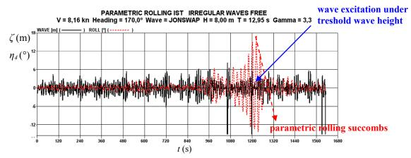
Figure 8-36. Wave elevation and roll time history of Test No. 36 with physical explanation
