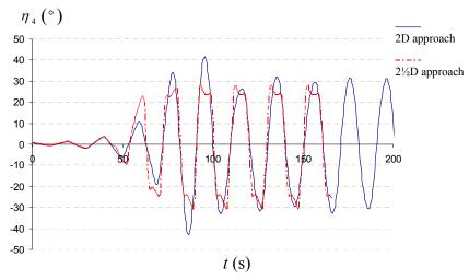
Figure 3-18. Nonlinear outlook of roll displacement with 2D and 2½D methods adopted
