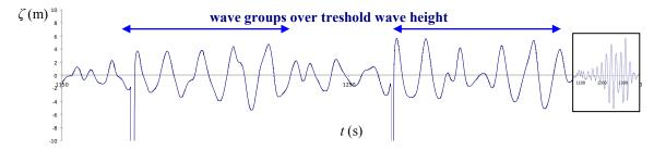
Figure 8-33. Segment of wave profile for which the parametric rolling initiates
