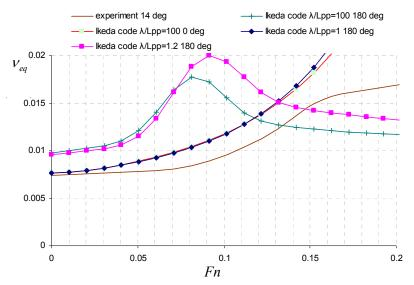
Figure 7-22. Equivalent linear damping  $v_{eq}(A)$  for 14° compared to numerical model
