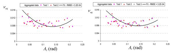
Figure 7-16. Linear + quadratic + cubic model for decay test by aggregating data (first 2 runs)
