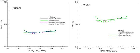
Figure 7-6. Dimensional roll damping evaluation by means of different methods (lin+quad)
