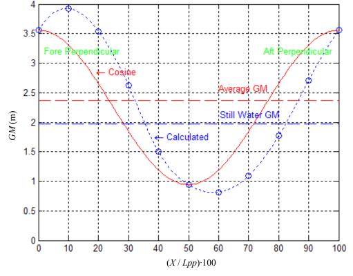
Figure 2-7. Wave-induced variation of the metacentric height GM (wave)
