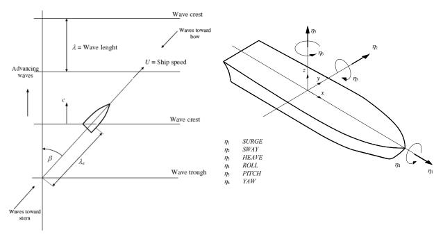
Figure 3-3. Coordinate system of incident harmonic wave Figure 3-4. Rigid body motions of the vessel
