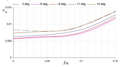
Figure 7-20 Equivalent linear damping  $\nu_{eq}\left(A\right)$  using the linear + quadratic + cubic model
