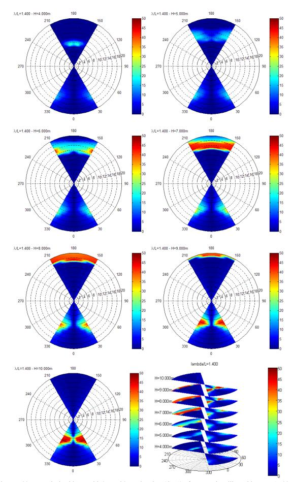
Figure 5-22. Numerical evidence with 2D and 3D polar plots (GM1) of parametric rolling with  $T_W = 15.33$  s.
