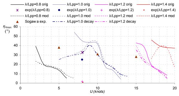
Figure 8-12. Numerical results of parametric roll with the roll damping estimated from a roll decay tests, Ikeda's method and modified damping feature with  $H_W = 8$  m
