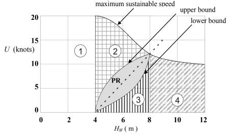
Figure 5-7. Risk of parametric as a function of significant wave height and sustained speed
