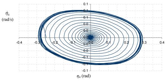
Figure 5-3. Phase diagram of the roll motion ( $H_W = 6 \text{ m}$ ,  $T_W = 12.95 \text{ s}$ , speed 7 knots)
