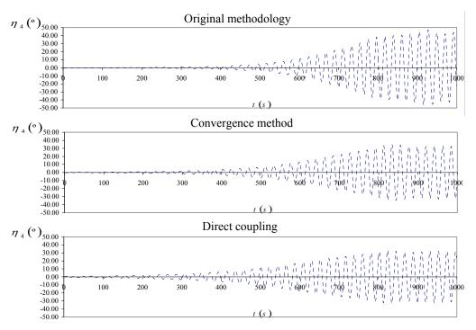
Figure 8-2. Time traces comparison of roll responses between the original methodology, convergence method and direct coupling for test No. 10
