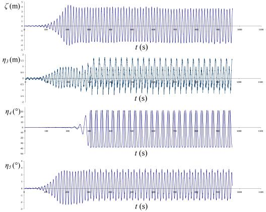
Figure 6-19. Experimental development of parametric rolling in experiments with regular following waves ( $H_W = 8 \text{ m}$ ,  $T_W = 12.95 \text{ s}$ , speed 0 knots)
