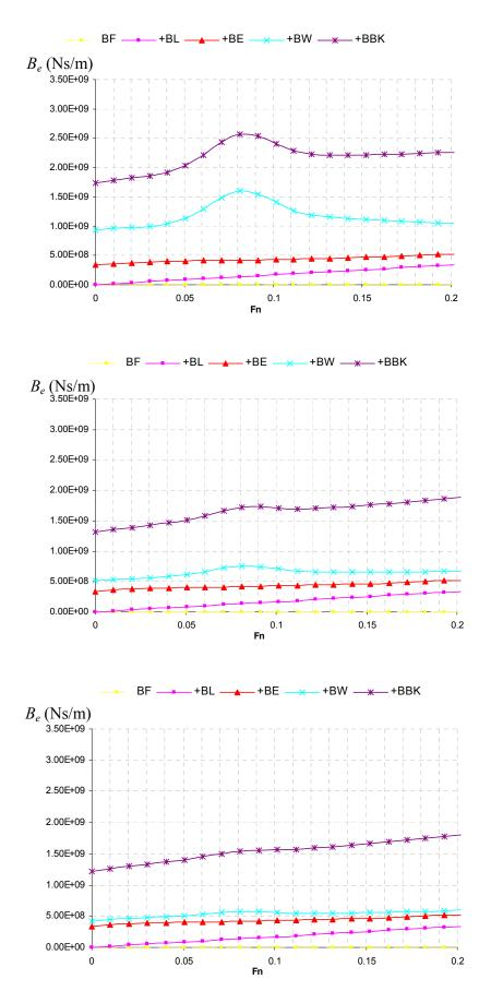
Figure 4-13abc. Comparison of the damping components for the 3 cases of wave radiation damping  $B_{w0}$  with the bilge keel with respect to velocity
