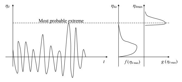
Figure 8-45. Assessment of roll extremes with small probability methodology
