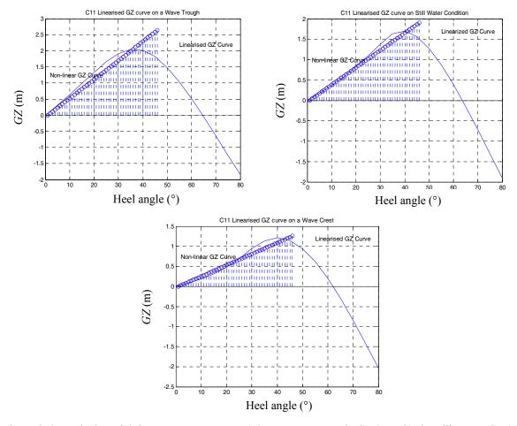
Figure 2-6. Equivalent righting arm curves up to  $45^{\circ}$  on a wave trough GZ (trough), in still water GZ (still) conditions, and on a wave crest GZ (crest) condition.
