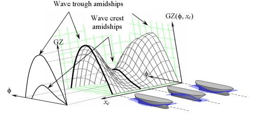
Figure 2-4. Schematics of the restoring moment as a function of wave position and heel angle, ABS (2004)
