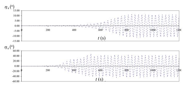
Figure 8-6. Time traces comparison of roll responses between numerical implementation and from the decay acquisition for test No. 310.
