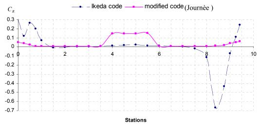
Figure 4-7. Roll damping distribution of coefficient  $C_R$  for original and modified methodology.
