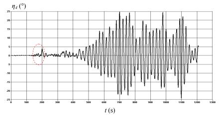
Figure 8-28. Experimental time trace of rolling motion for Test No. 26.
