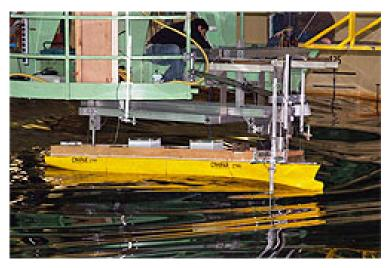
Figure 6-3. Experimental setup for the parametric rolling tests
