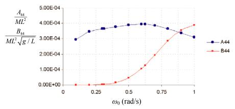
Figure 3-13. Added mass and damping coefficients of roll motion (Ribeiro e Silva et al. 2005.)
