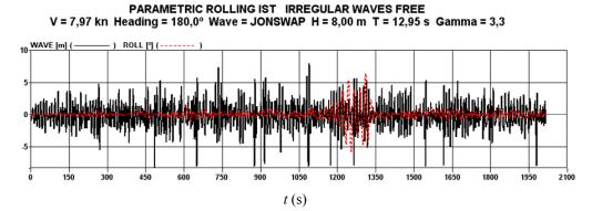
Figure 8-32. Wave elevation and roll time history of Test No. 35
