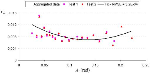
Figure 7-14. Linear + quadratic + cubic model for decay test "DECAY\_TEST\_GM1\_ U=0 knots" by aggregating data from both runs
