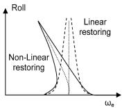
Figure 3-21 Nonlinear effects of restoring.
