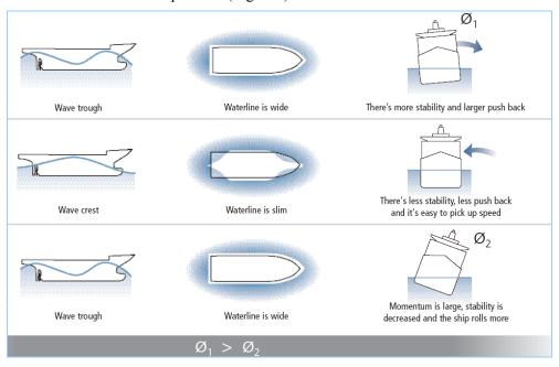
Figure 2-3. Schematic representation of a hull contact with the sea, with respect to beam changes as a cause of parametric roll resonance.
