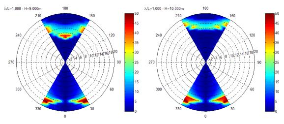
Figure 5-18. Numerical evidence with polar plots (GM1) of parametric rolling for ( $H_W = 9/10 \text{ m}$ ,  $T_W = 12.95 \text{ s}$ ).
