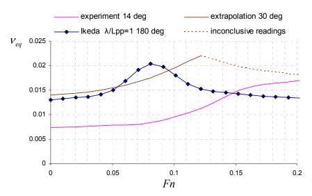
Figure 7-23. Equivalent linear damping  $v_{eq}(A)$  for 30° compared to numerical model
