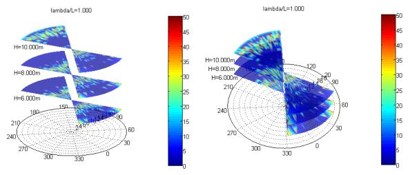
Figure 8-50. Numerical evidence with 3D polar plots of parametric rolling with irregular following waves ( $T_Z$  = 12.95 s).
