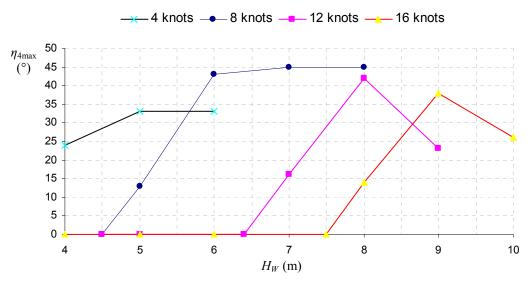
Figure 5-11. Linear fitting for varying speeds with roll responses as a function of wave heights
