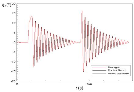
Figure 6-11. Time trace of decay test for 0 knots with filtering
