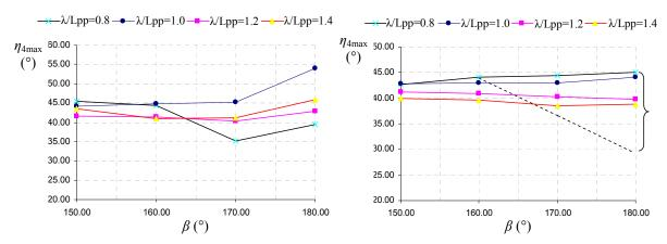
Figure 5-13. Comparison of roll response from both original and modified methodology for different headings
