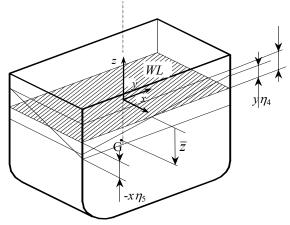
Figure 3-6. Displacement caused by coupling of the heave, roll and pitch motions
