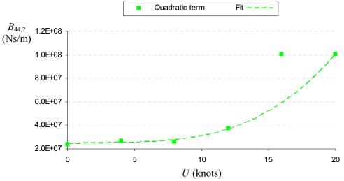
Figure 7-12. Evalution of the quadratic component of damping for all speeds using decay tests 302 to 307
