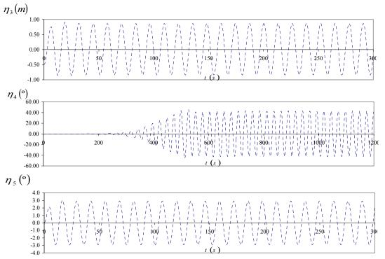
Figure 8-1. Numerical development of parametric rolling with regular following waves ( $H_W = 8 \text{ m}$ ,  $T_W = 12.95 \text{ s}$ , speed 0 knots)
