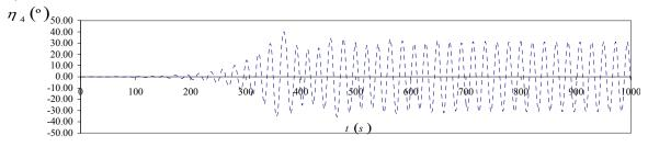
Figure 8-3. Time traces of roll responses with linear + quadratic damping model from decay test No. 304
