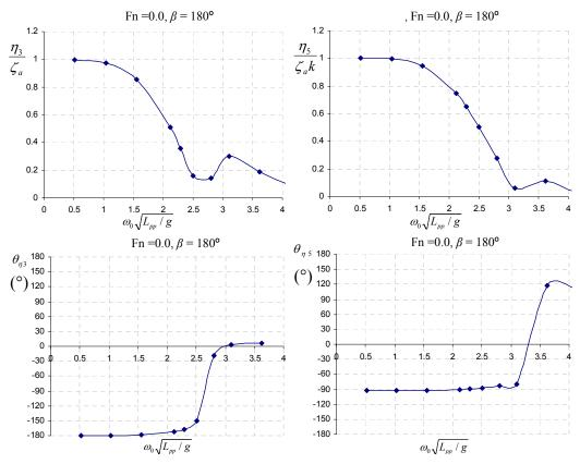
Figure 3-7. Transfer functions for C11 containership in heave and pitch in head seas at zero speed
