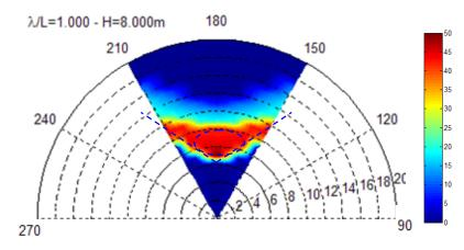
Figure 8-17. Speed increase for slightly oblique waves due to the established occurrence groupiness.
