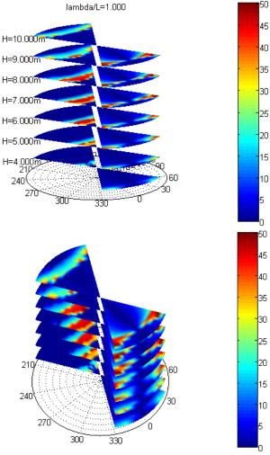
Figure 5-19. Numerical evidence with 3D polar plots (GM1) of parametric rolling with  $T_W = 12.95 \text{ s}$ .
