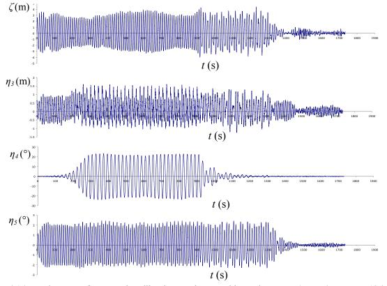
Figure 6-16 Development of parametric rolling in experiments with regular waves ( $H_W = 6 \text{ m}$ ,  $T_W = 12.95 \text{ s}$ , speed 8 knots)
