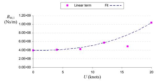
Figure 7-11. Evalution of the linear component of damping for all speeds using decay tests 302 to 307
