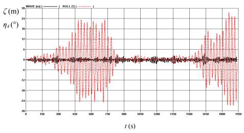
Figure 8-42. Wave elevation and roll time history of Test No. 341.
