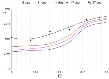
Figure 7-21. Equivalent linear damping  $\nu_{eq}(A)$  using the linear + quadratic + cubic model up to 17°
