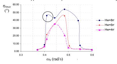
Figure 5-5. Regular wave parametric roll response for C11-class ship (original methodology)
