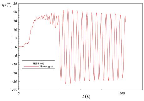
Figure 6-15. No damping for decay test 469
