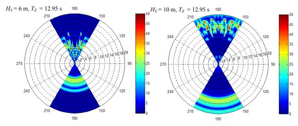
Figure 8-48. Weighted generalization of the irregular parametric excitation for  $(H_S = 6 \text{ and } 10 \text{ m}, T_Z = 12.95 \text{ s})$ .
