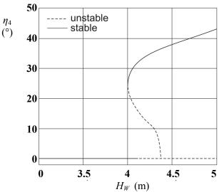
Figure 5-8. Stable and unstable realizations of roll responses
