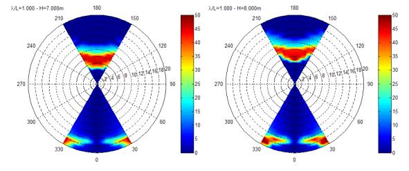
Figure 5-17. Numerical evidence with polar plots (GM1) of parametric rolling for ( $H_W = 7 / 8$  m,  $T_W = 12.95$  s).
