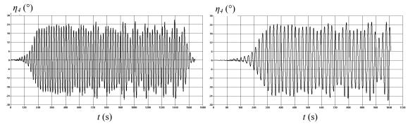
Figure 8-19. Experimental time trace of rolling motion for Test No. 23 and Test No. 25. provided by Cehipar
