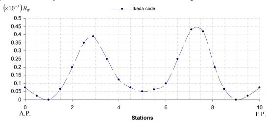
Figure 4-2. Roll damping distribution of wave component.
