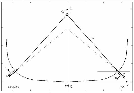
Figure 4-11. Geometry for calculating sectional damping coefficient due to normal force of the anti-roll fins.
