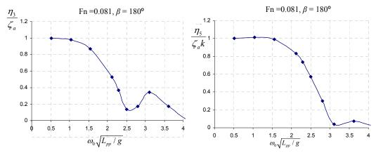
Figure 3-8. Transfer functions for C11 containership in heave and pitch in head seas for 8 knots
