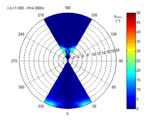
Figure 5-15. Numerical evidence with polar plots (GM1) of parametric rolling for ( $H_W = 4$  m,  $T_W = 12.95$  s).
