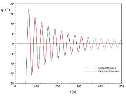
Figure 7-8. Comparison between time series from experiment and time series obtained by Runge Kutta method
