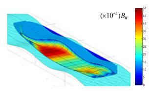
Figure 4-3. Simulated 3D roll damping distribution of wave component.
