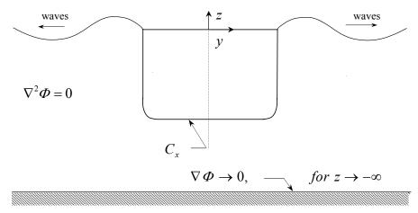
Figure 3-5. Radiation condition on a two dimensional strip
