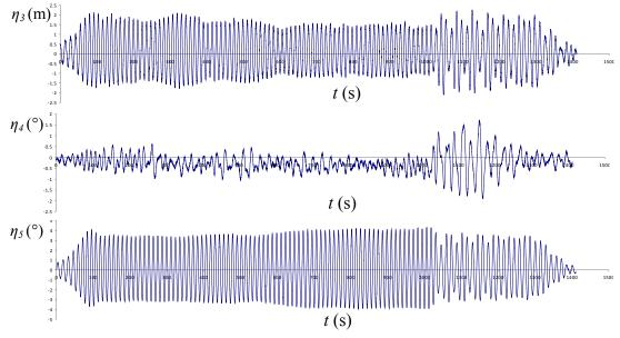
Figure 6-18. No parametric rolling in experiments with regular waves ( $H_W = 8 \text{ m}$ ,  $T_W = 14.19 \text{ s}$ , speed 8 knots)
