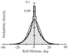
Figure 8-44. Distribution of parametric roll
