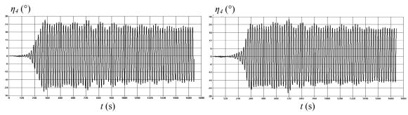
Figure 8-16. Experimental time trace of rolling motion for Test No. 18 and Test No. 19. provided by Cehipar
