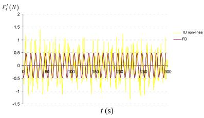
Figure 3-15. Linear and nonlinear simulation of Froude-Krylov force in roll
