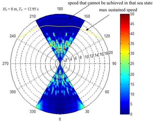
Figure 8-47. Numerical evidence with polar plots of parametric rolling for  $(H_S = 8 \text{ m}, T_Z = 12.95 \text{ s})$ .
