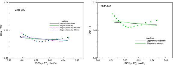
Figure 7-4. Dimensional roll damping evaluation by means of different methods (lin+quad)
