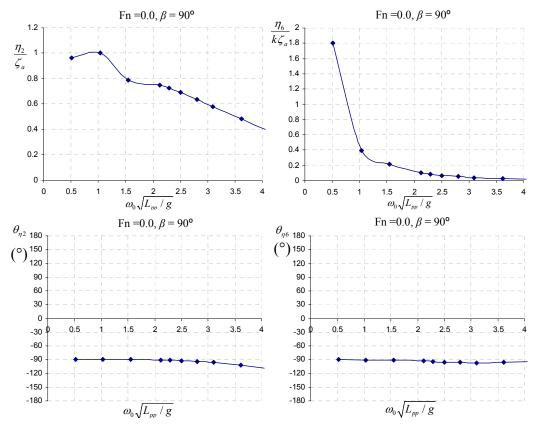
Figure 3-9. Transfer functions for C11 containership in sway and yaw in beam seas at zero speed
