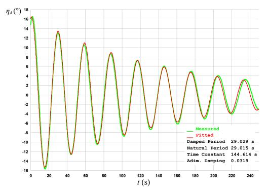
Figure 7-9. Decay test 302 processed by the exponential fitting method
