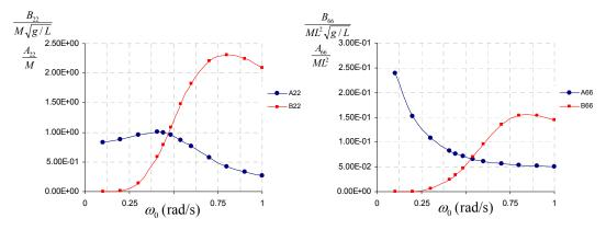
Figure 3-12. Variations of the hydrodynamic added mass and damping coefficients in sway and yaw depending on the various encounter frequencies
