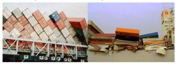
Figure 1-1. Casualties due to the parametric rolling on APL China.
