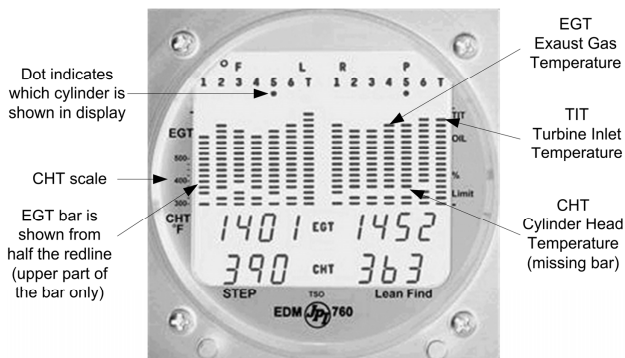
Figure 1. Engine monitor display (EDM 760) for twin-engine aircraft
