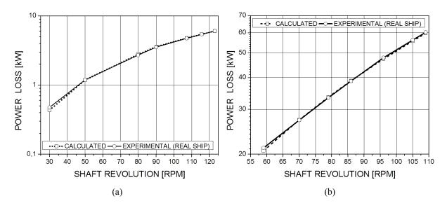
Fig. 6 Comparison of the theoretical and experimental calculation of the power loss in aft stern tube white metal bearing at various shaft revolutions and constant bearing load: (a) bulk carrier of 50000 DWT, bearing load of 225 kN; (b) container ship of 11000 TEU, bearing load of 1325 kN.
