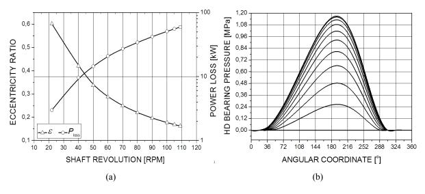
Fig. 3 Calculated relationship between significant parameters of the stern tube white metal bearing in steady state condition with constant radial load of 1325 kN at various shaft revolutions:(a) power loss versus eccentricity ratio, (b) bearing pressure field at 109 rpm of the propeller shaft
