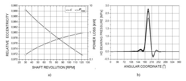
**Fig. 4** Calculated relationship between significant parameters of the stern tube with polymer bearing in steady state condition with constant radial load of 225 kN at various shaft revolutions as follows: (a) power loss versus eccentricity ratio, (b) bearing pressure field at 121 rpm of the propeller shaft.
