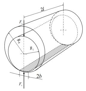
Fig. 1 Geometry of the contact area between the journal and the bearing
