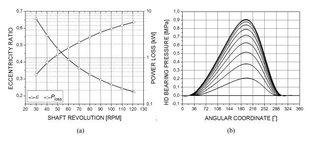
Fig. 2 Calculated relationship between significant parameters of the stern tube white metal bearing in steady state conditions with constant radial load of 225 kN at various shaft revolutions: (a) power loss versus eccentricity ratio, (b) bearing pressure field at 121 rpm of the propeller shaft.
