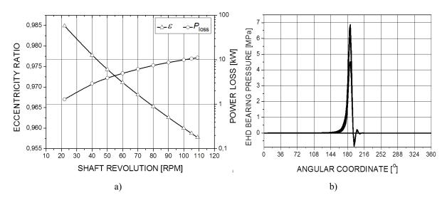
**Fig. 5** Calculated relationship between significant parameters of the stern tube with polymer bearing in steady state condition with constant radial load of 1325 kN at various shaft revolutions as follows: (a) power loss versus eccentricity ratio, (b) bearing pressure field at 109 rpm of the propeller shaft
