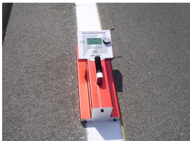
Fig. 1. Device for measuring retroreflection of road markings Source: Prepared by the authors
