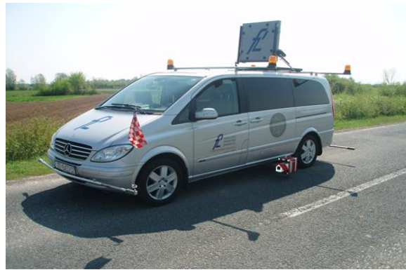
Fig. 5. Measurement vehicle with dynamic retroreflector Source: Prepared by the authors
