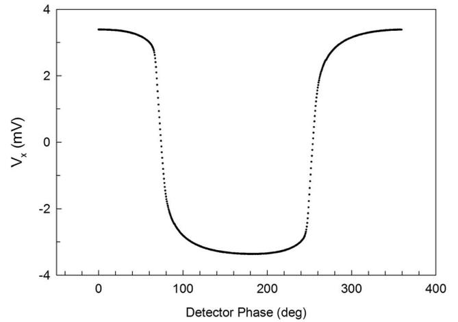
FIG. 4. Voltage measured in first channel of PAR 5210 lock-in (in FLAT mode) as the function of lock-in phase.
