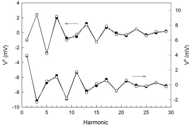
FIG. 3. RMS amplitudes of real (down) and imaginary (up) Fourier components of induced voltage obtained from fit of digitized voltage (full dots) and directly measured on Ametek 7265 lock-in (empty dots).
