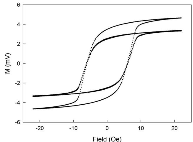
FIG. 5. Hysteresis obtained by: integration of digitized induced voltage (elongated one), constructed from 50 harmonics measured by Ametek 7265, and directly measured by PAR 5210 lock-in. Latter two almost coincide.
