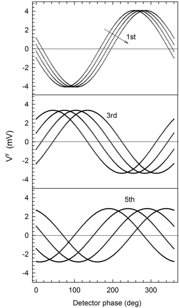
FIG. 2. 1st, 3rd, and 5th even component of induced voltage for arbitrary source phase and phase shifted for  $10^\circ$ ,  $20^\circ$ , and  $30^\circ$  as a function of detector phase. Arrow shows shift of source phase, same for all three harmonics.
