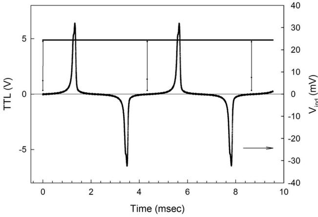
FIG. 1. Voltage induced in secondary coils and corresponding TTL signal as function of time.
