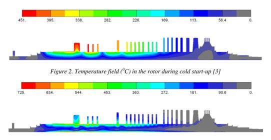
Figure 3. HMH stresses (N/mm<sup>2</sup>) in the rotor during cold start-up [3]
