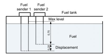
*Figure 3* Fuel tank with two capacitive fuel senders submerged to different depths (the diameter of fuel senders is enlarged in comparison with the tank for clarity purpose)
