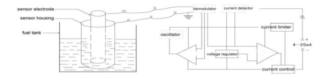
Figure 2 Fuel level sensor schematic
