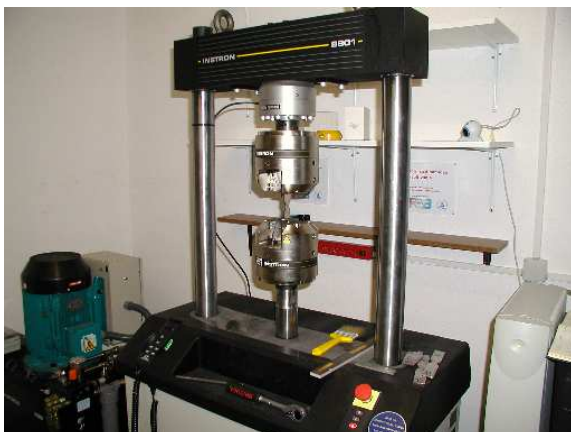
Fig. 7 Servo hydraulic testing machine INSTRON 8801
