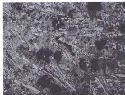
Fig. 12. Hardness drop and metallographic structure (500 ×).
