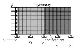
**Fig. 2.** Axis-symmetric computational domain and the schematic of the finite element mesh for the FEM analysis
