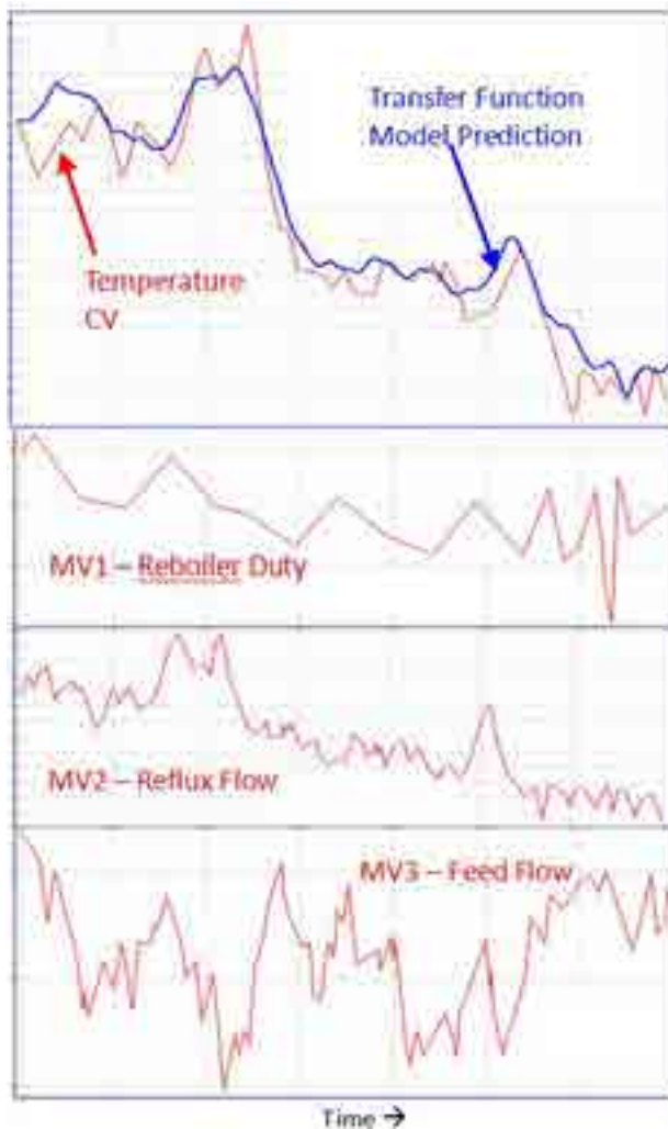
Figure 7: Simultaneous multi-input closed-loop process model parameters identification with short duration data and no pulse tests
