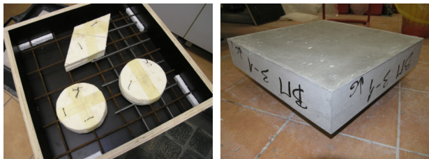
Figure 4 Concrete test specimen with polystyrene defects, preparation stage and finished specimen
