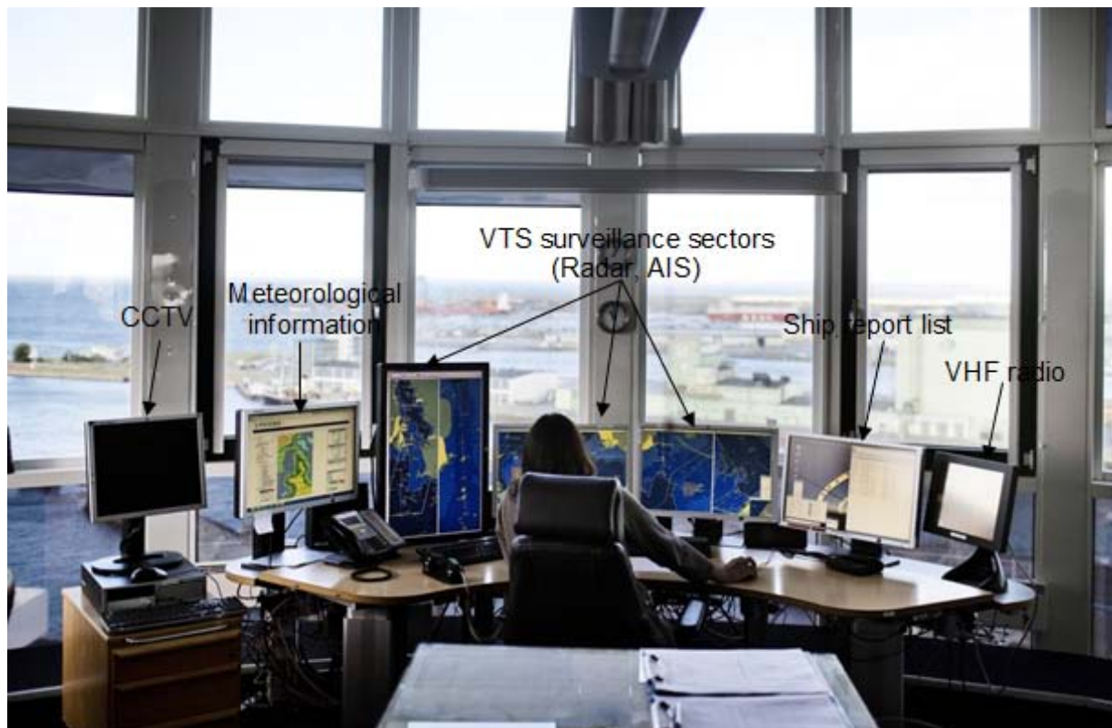
Figure 3. Overview of the VTS working place Source: Authors
