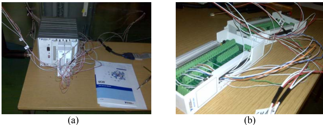
Figure 6. The National Instruments SCXI data acquisition system (a) and National Instruments DAQCard (b)
