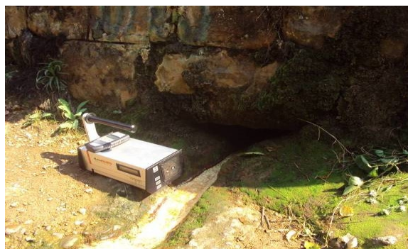
Figure 1. Placement of the measuring instrument at the research sites, AlphaGuard placed near the source (Voda Ljepotica-Srebrenica)
