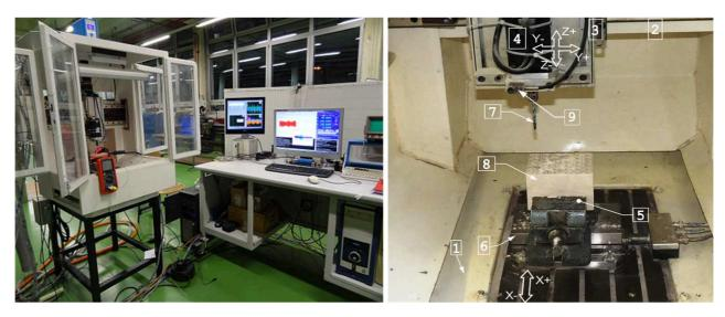
Fig. 1. Experimental setup - work area and sensor placement. (1) X axis feed drive; (2) Y axis feed drive; (3) Z axis feed drive; (4) main spindle drive; (5) workpiece fixture; (6) three axis force sensor; (7) test drill; (8) stone workpiece; (9) AE sensor
