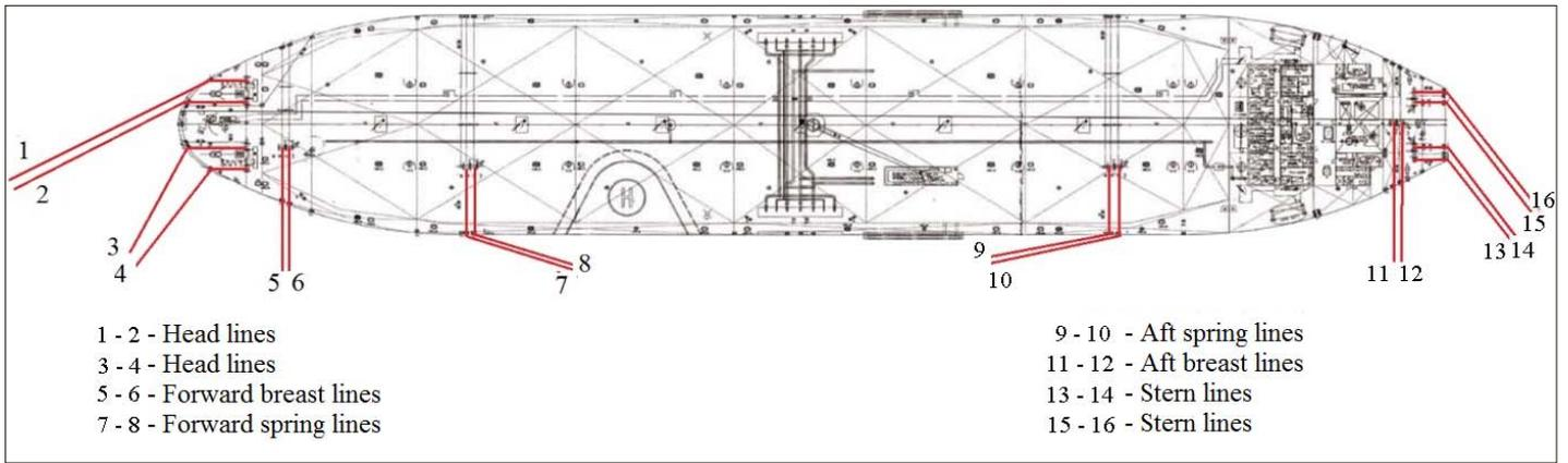
Figure 3. Vessel mooring ropes by location
