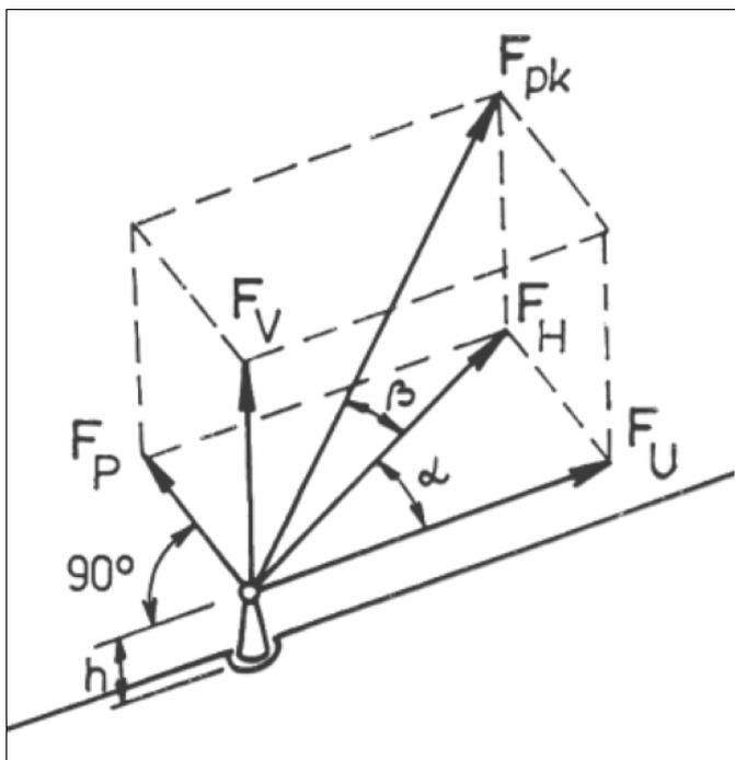
Figure 4. Components of mooring ropes angles
