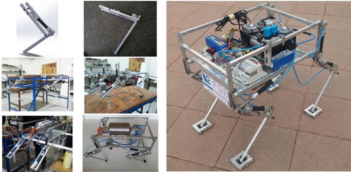
Figure 4: Construction process of WRAPAM and its final form
