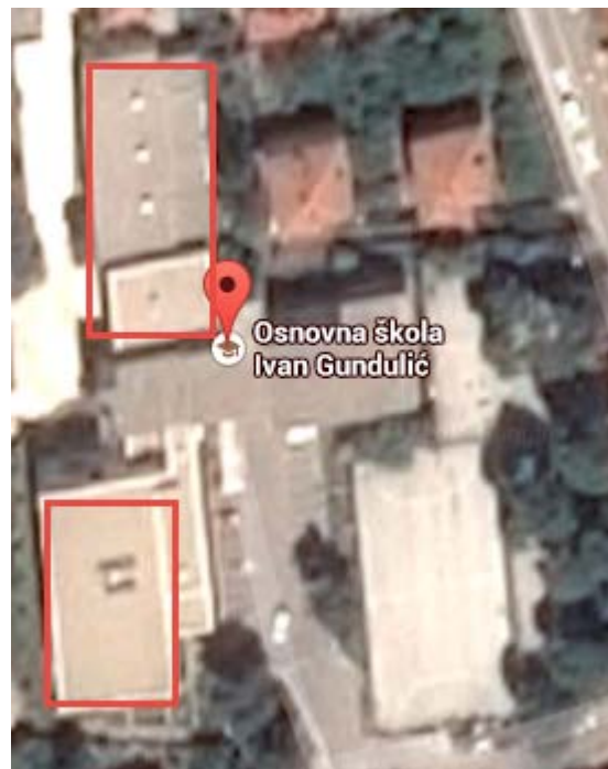
Picture 2. Area of roof reserved for solar thermal collector field
