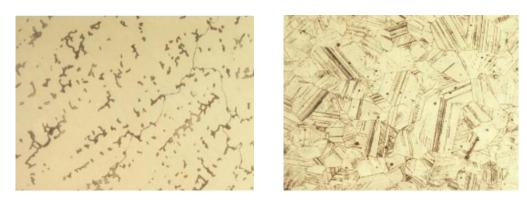
**Figure 2.** Microstructure of as cast and wrought Co-Cr-Mo alloy, 200x [11] **Figure 2.** Mikrostruktura lijevane i kovane Co-Cr-Mo slitine, 200x [11]
