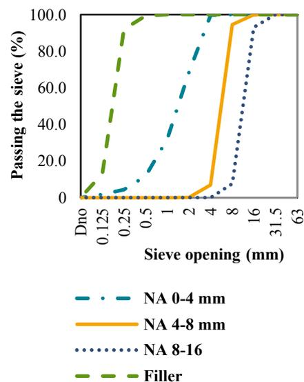
**Figure 1.** Grading curves for dolomite.
