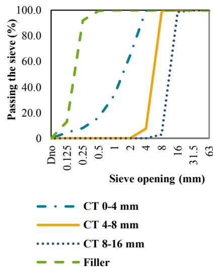
Figure 2. Grading curves of crushed roof tiles.
