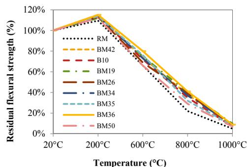
Figure 13. Residual flexural strengths.
