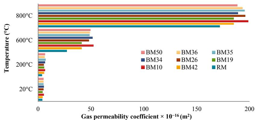
Figure 16. Gas permeability after exposure to high temperatures.
