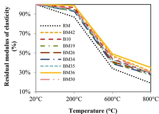
Figure 14. Residual modulus of elasticity.
