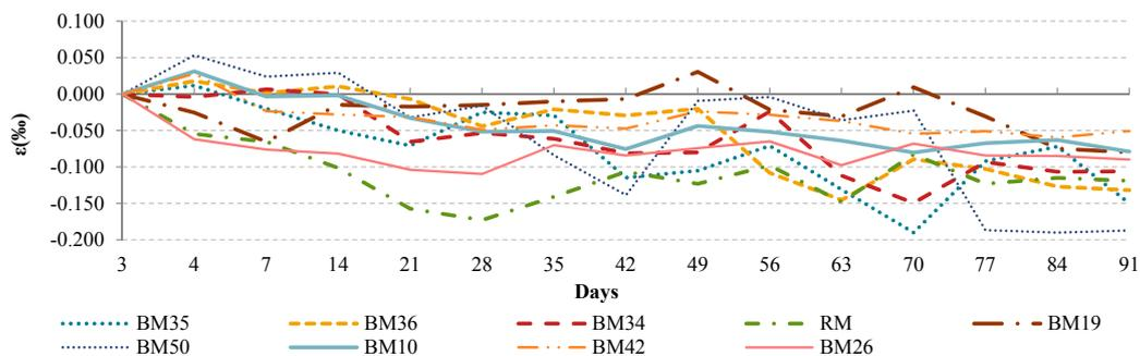
**Figure 4.** Comparison of drying shrinkage of concrete mixtures.
