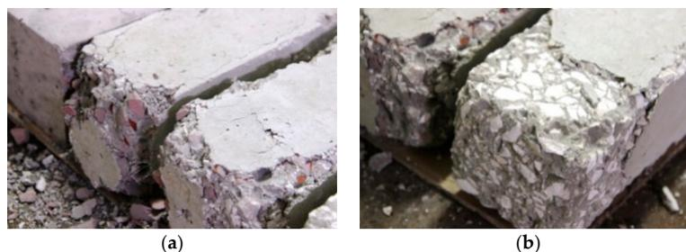
Figure 17. Examples of fire spalling of concrete surface after exposure to a temperature of 1000 °C for different concrete mixtures. (a) Concrete with CB and CT aggregates; (b) Mixture RM.
