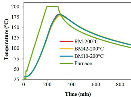
Figure 8. Heating regime of mixtures RM, BM10 and BM42 for 200 °C.
