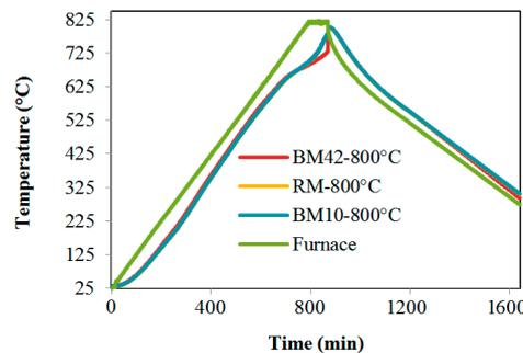
Figure 9. Heating regime of mixtures RM, BM10 and BM42 for 800 °C.
