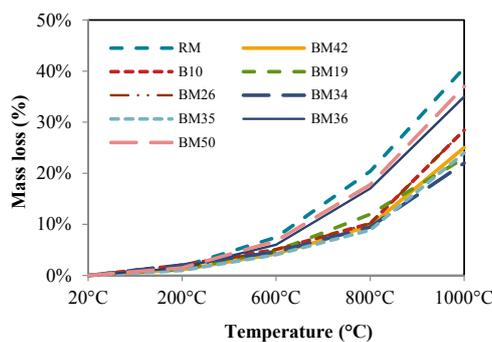
Figure 10. Mass loss after exposure to high temperatures.
