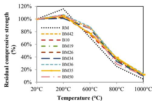
Figure 12. Residual compressive strengths.
