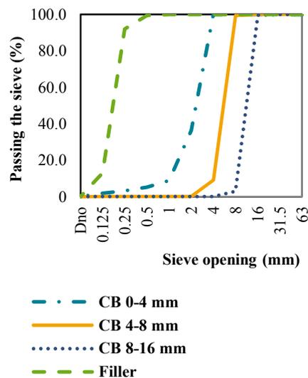
Figure 3. Grading curves of crushed bricks.
