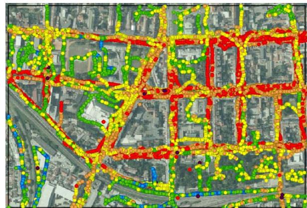
Figure 8. Classified measurements displayed in QGIS (blue and green dots represents lowest noise levels, red and purple the highest) (Vuković, 2015)
