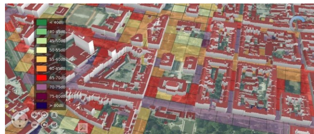
Figure 4. Dynamic noise map on the web platform with a 3D model
