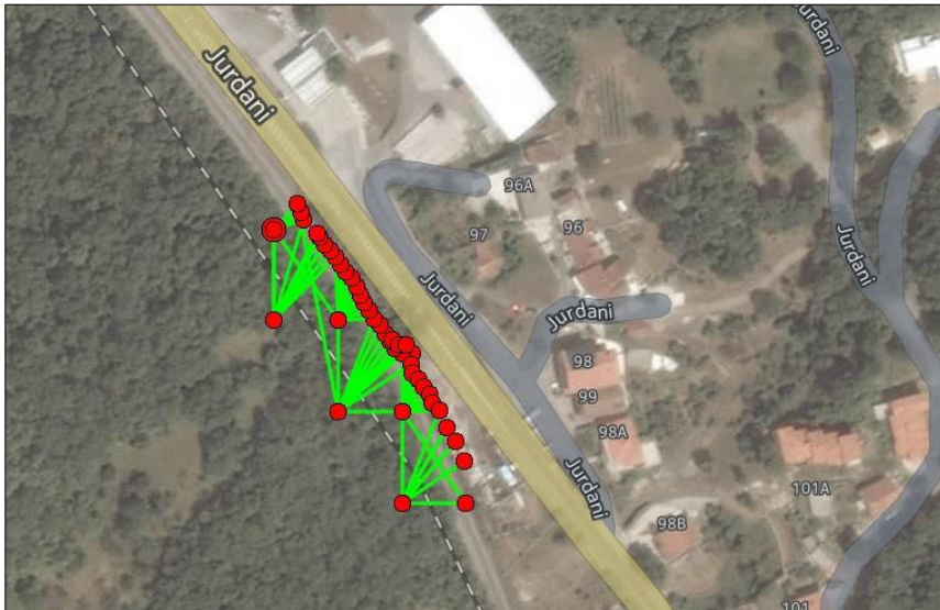
Figure 5. Screen shot of Pix4D mapper Pro with positions where images were taken
