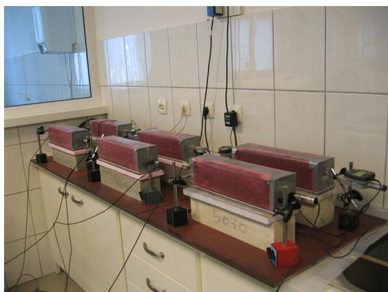
Fig. 1 Measuring initial autogenous shrinkage of concrete specimens.
